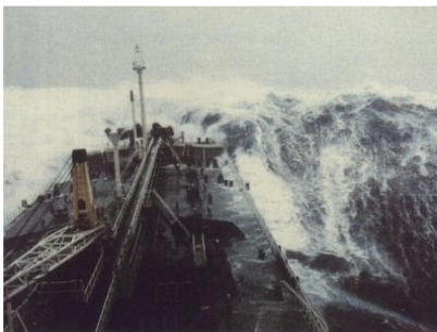
BEAUFORT FORCE 12 WIND SPEED: 64 KNOTS SEA: SEA COMPLETELY WHITE WITH DRIVING SPRAY, VISIBILITY VERY SERIOUSLY AFFECTED. THE AIR IS FILLED WITH FOAM AND SPRAY
